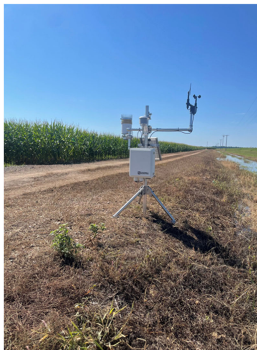
Mobile Weather Station at a Corn Variety Trial At Money, Mississippi 2024
