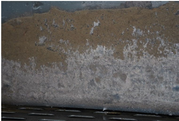
Figure 2: Marietta Fine Sandy Loam after receiving its first ¼ inch showing the water infiltration observed percolating through the soil profile.
