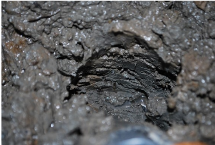
Figure 1: Sharkey Clay after receiving 0.8125 inches (13/16 inches) in 800 seconds (13 minutes and 20 seconds) showing saturation down to
